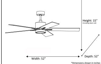
**ELECTRICAL REQUIREMENTS:** Fixture requires a grounded electrical supply line of 120 volts AC.
